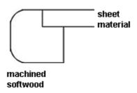
Right shows a sectional view of the machined softwood used to support the front of a shelf made from sheet material.
