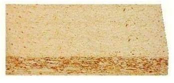
surface. Chipboard is available in a number of densities; normal, medium and high-density. Normal density is fairly soft and 'flaky', high-density is very solid and hard (often used for worktops and fire doors) - medium density is somewhere in between.
