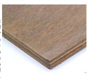
the stronger the plywood. Both the type of glue and veneers determine the suitability of a sheet for a particular application. The finish quality of plywood varies enormously, some have attractive grains while others can have a large number of knots.
